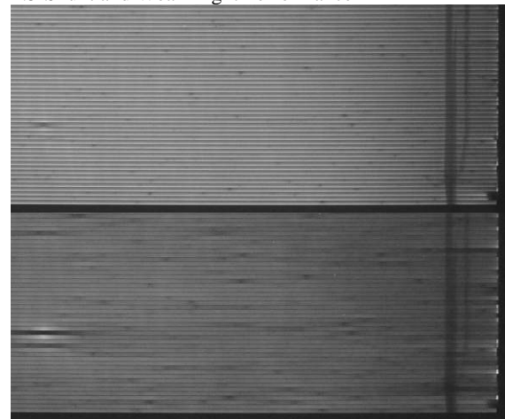
Figure 5: EL pictures of a part of a CIGS module (Y). The upper image (A) has been recorded using an injection current density of J = 40 mA/cm 2 and for the bottom (B) image J = 10 mA/cm 2 has been applied. “A” reveals many shunts shown as dots, whereas “B” shows a pronounced quenching of the EL signal around the shunts.
