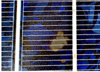
**Figure 4:** Permanent “hot spot” at a solar cell (light grey area in the center).
