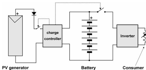
**Figure 1:** Scheme of a typical autonomous PV system with a single-phase AC outlet, including PV generator, energy storage, charge controller and DC-AC converter (inverter).
