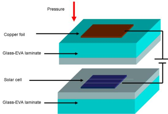
Figure 1: Schematic test-setup with two glass-EVA laminates and a crystalline silicon cell in between. Both glass plates have been pressed together to simulate a laminated module. The outside surface of the front glass has been equipped with copper foil. The foil and the cells contacts have been connected to a laboratory DC power supply and have been stressed with a voltage of -200V at 50°C at 20% RH.
