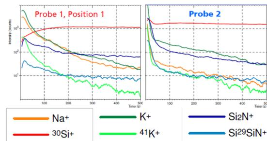
Figure 3: TOFSIMS profiles of a polarized cell (Probe 1) and an unaffected reference cell (Probe 2) for various elements.
