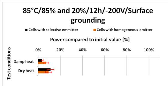
Figure 4: PID susceptibility comparison of crystalline silicon cells with selective and homogenous emitter. Both test runs, at damp heat (85°C/85%RH) and dry heat (85°C/20%RH) conditions, showed no significant differences between both cell concepts.
