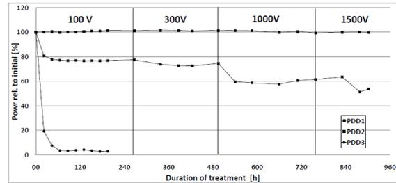
Figure 8: The susceptibility to PID varies significantly over a wide range of modules. Some modules show a rapid loss in performance at a very low voltage level (PDD3) whereas other modules don't even show degradation tendencies at voltages beyond the 1000V mark (PDD1). A voltage dependency could be determined as shown with PDD2, which shows a saturation state at every voltage level.
