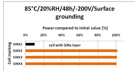
Figure 2: Cells without  $\text{SiN}_x$ -ARC show no degradation of performance due to PID stress test.
