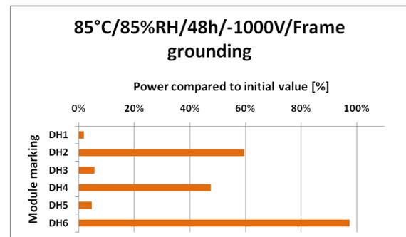
Figure 6: After adding humidity to the test sequence all modules show power distributions. The mismatch between the modules becomes significant for each module type.
