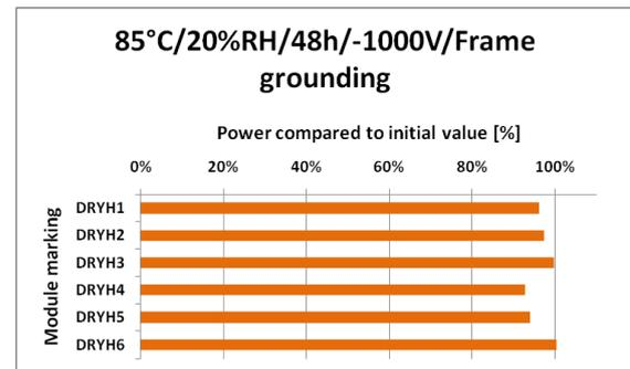
Figure 5: Nearly no power distribution was determined after 48 hours stress test with a relative humidity of 20%. Only a slight mismatch between the single module types is observed.
