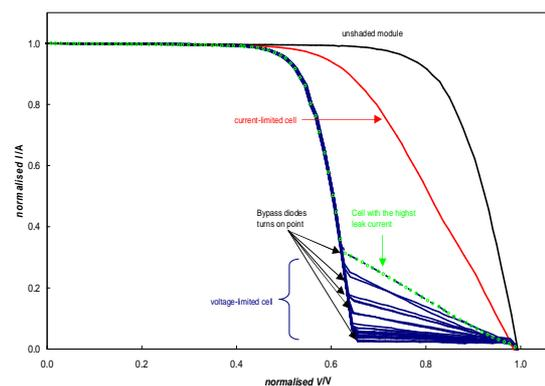
**Figure 2:** The shaded cell is reversed bias by the unshaded cells. Bypass diodes are used to reduce the reverse bias voltage and with this the power dissipation.
