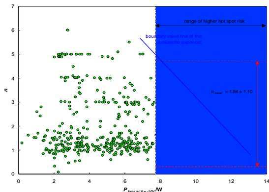
**Figure 5:** The avalanche exponent  $n$  vs. dissipated power for 420 different shaded cells.
